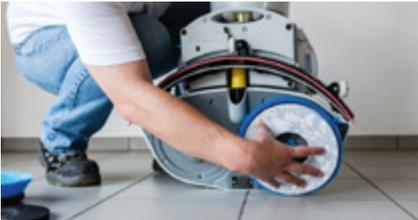
Mount the traction plates against the direction of travel until they engage.
