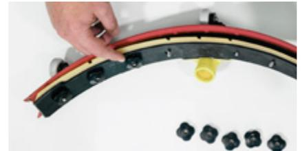
Loosen the screw connections of the suction bar.
