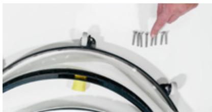
Replace the worn suction lip with a new one. Note the different lengths of the screws.
